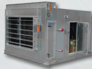
Fig. 4 - Air handling unit utilizing return and outside air with louvers, an access door, a steam coil, another access door and a blower/motor arranged in series. The bolting pattern around the louvers are designed to meet with an existing duct, and the access doors provide a convenient way to conduct maintenance on all components of the air handling unit.
