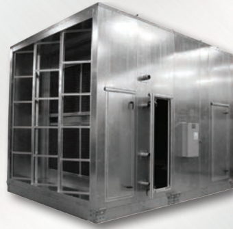
Fig. 2 - Welded housing unit with a filter bank, access door, two steam coils, stacked on top of each other, and two more access doors arranged in series. The access doors ease the process of replacing the filters and inspecting and cleaning of the coils.
